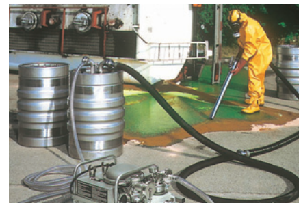
Recovery Pump (流出油回収装置)
