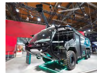
EV airport chemical fire engine
