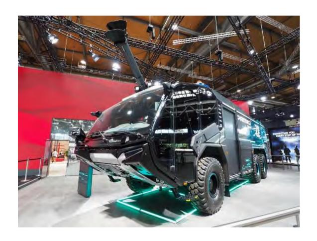
◆ EV airport chemical fire engine made by Rosenbauer
